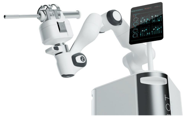
Figure 1. Rendering of the mechanical structure of the PROST robot. The system is composed of a support arm that moves the robotic head. The robotic head allows the orientation of the needle and the movement of the US probe. US, ultrasound.
