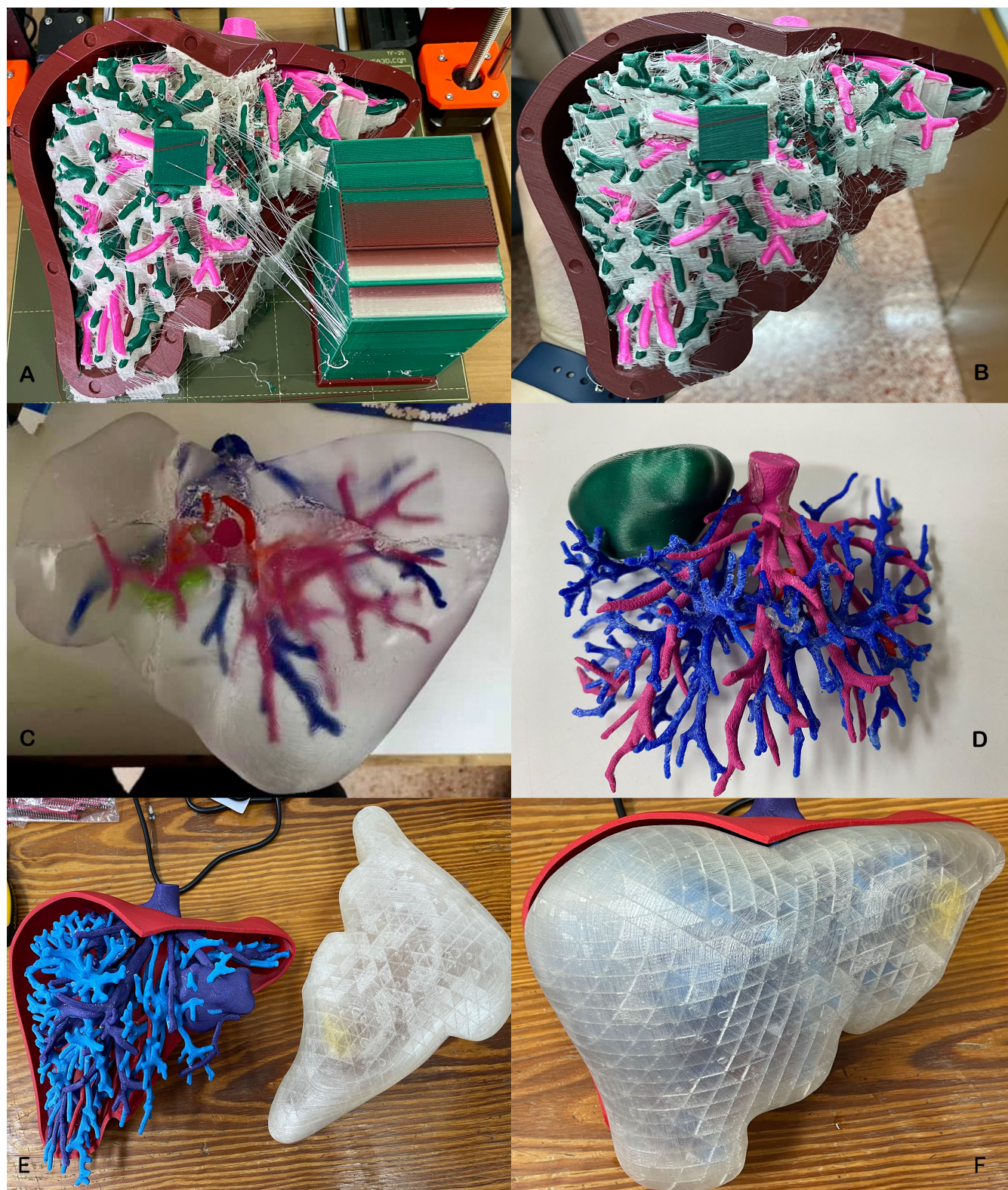
Figure 2. 3D printed model with fused deposition modeling technology combined with Mosaic Pallette 2s machine. pink: hepatic vein, green: portal vein, red: liver parenchyma and arteries, white: supportive structure. A. 3D model inside the printer. B. 3D model outside the printer. C. 3D liver model with fused deposition model technology and resin fill. D. Previous model before the resin-fill. E and F. 3D liver model with fused deposition model technology. blue: portal vein; purple: hepatic vein and liver tumor; red: hepatic artery and liver parenchyma; the transparent segment represents half of the hepatic parenchyma and complements the rest of the model.
